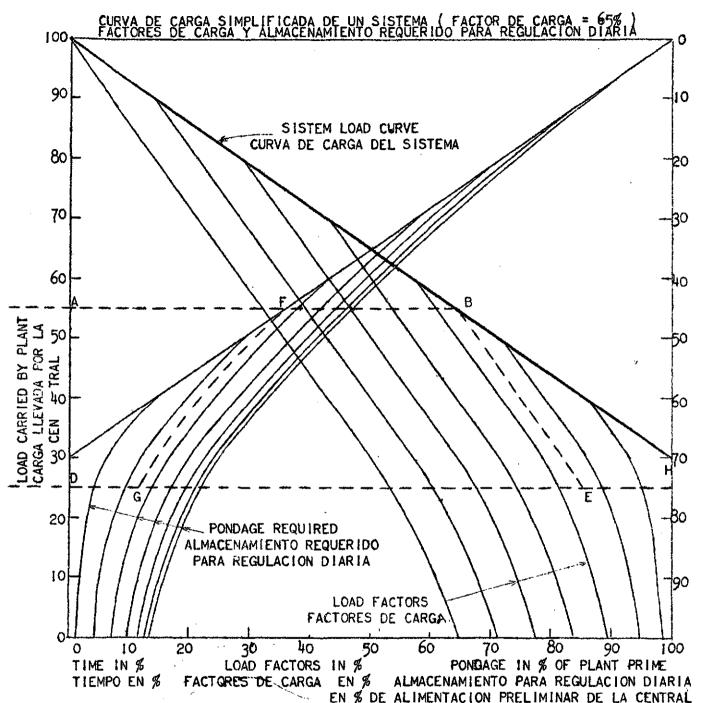
ASSUME HYDRO PLANT ALLOCATED TO LOAD COMPRISED BETWEEN HORIZONTAL LINES AB & CD PLANT LOAD FACTOR IS SHOWN BY INTERPOLATING ALONG LINE BE, OR ABOUT 85 % PONDAGE REQUIRED IS SHOWN BY INTERPOLATING ALONG FG, OR ABOUT 12 % OF PLANT PRIME, 1E, ABOUT 12 % OF ENERGY IN LOAD CURVE BETWEEN LINES AB & CD
